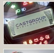
Electronic display with warning lights indicating faults, engine, hydraulic oil gauge, and electric floating system.
