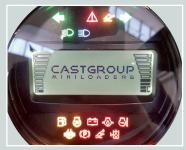
Electronic display with warning lights indicating faults, engine, hydraulic oil gauge, and electric floating system.
