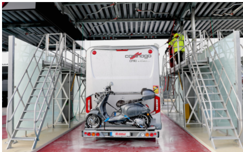
Steel construction Waschheld Easy access for roof cleaning
