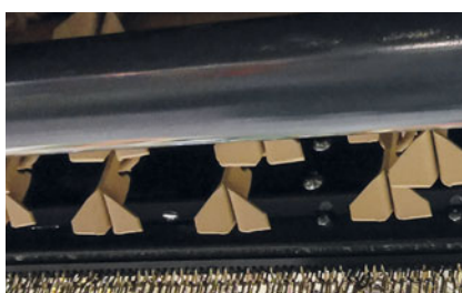
Polyurethane-coated support rollers
