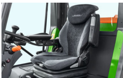
Various seat options, such as the Grammer "De Luxe" seat with air suspension and heating
